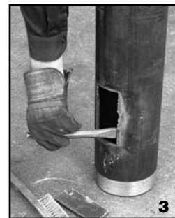
Remove slag and burrs.
